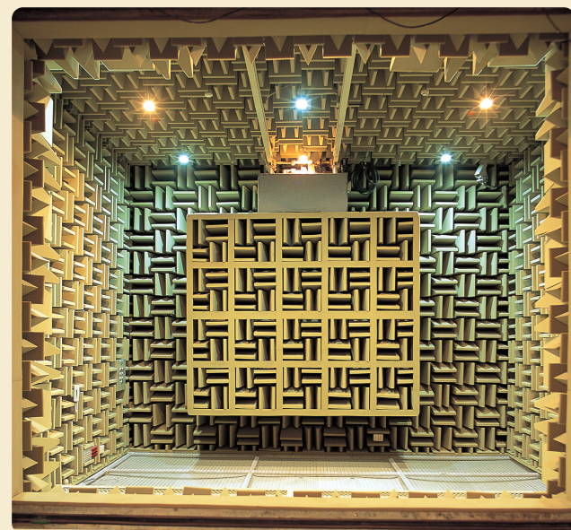
▶ 무향실 (Anechoic Chamber)
